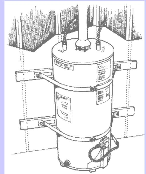
**Typical gas water heater with earthquake straps.**
